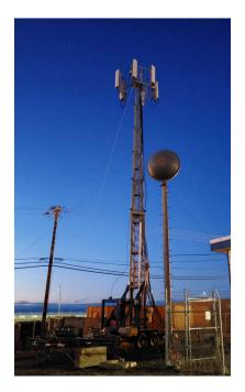
Backhaul delivery to the network can be via terrestrial microwave, communication satellite or existing wired infrastructure. The COW can be transported over large distances and on rough terrain and may be left on site for an extended period of time with the use of either mains power or a backup generator.
